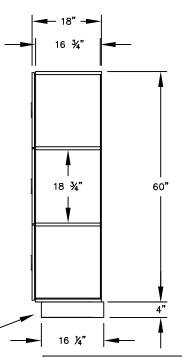
(BASES ARE MADE OF INDUSTRIAL GRADE PARTICLEBOARD AND ARE COVERED IN A DURABLE BLACK LAMINATE. PLEASE SET BASE TO ALLOW %" BETWEEN THE BACK OF THE LOCKER AND THE WALL FOR AIR VENTILATION.)
