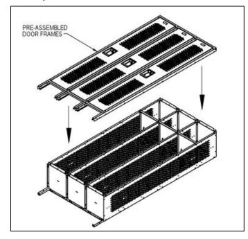
**Step 9:** Tighten all fasteners checking for squareness of the locker while tightening. Attach optional sloping hoods, end bases or front bases (see pages 4 and 5).
