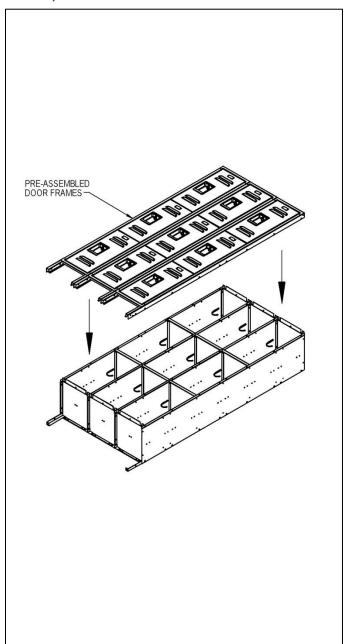
**Step 9:** Tighten all fasteners checking for squareness of the locker while tightening. Attach optional sloping hoods, end bases or front bases (see pages 4 and 5).
