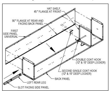
**Step 3:** Attach the second side panel and the right rear leg to the assembly of Step 2. On 12" and 15" deep lockers attach a third single coat hook. On 18" deep lockers substitute a single coat hook with a double bend for the third single coat hook and install the coat rod as shown on page 3. The locker chassis is now complete.
