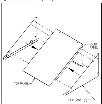
Step 3: Attach the sloping hood to the top of the locker with #10 - 24 x 3/8" slot less screws and #10 nuts (provided).
