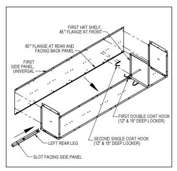
**Step 3:** Attach the second top shelf, the second bottom shelf, and an additional single coat hook to the second back panel as in step 1.
