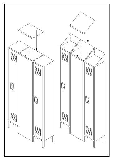
As an alternate method, the 15" wide top filler may be used to cover any gap or front filler width smaller than 15" without trimming the top filler width as shown in the illustration below. Simply use the full width top filler as is and place it into a position straddling the smaller opening between locker tops.
