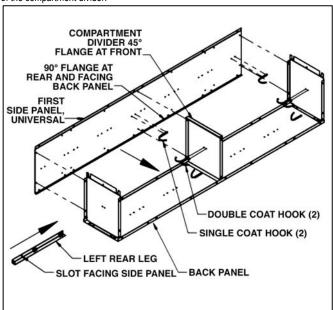
**Step 3:** Attach the second side panel and the right rear leg to the assembly of Step 2. Attach an additional two single coat hooks to the second side panel. The locker chassis is now complete.
