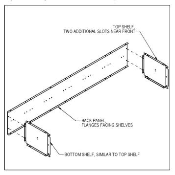
**Step 2:** Turn the back panel on its back with the shelves pointing upward. Attach the first side panel, the left rear leg, and three compartment dividers to the assembly from Step 1.
